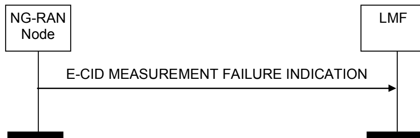
Figure 8.2.2.2-1: E-CID Measurement Failure Indication, successful operation
