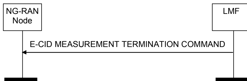
Figure 8.2.4.2-1: E-CID Measurement Termination procedure, successful operation
