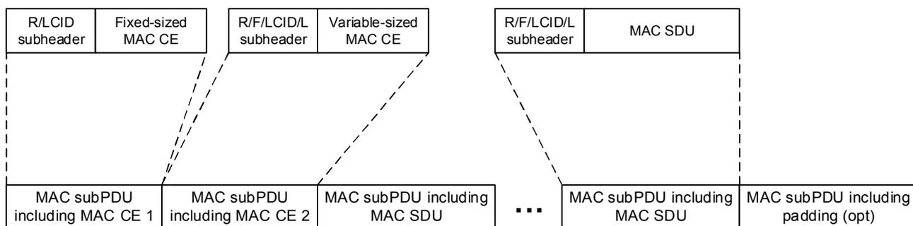
Figure 6.1.2-4: Example of a DL MAC PDU
