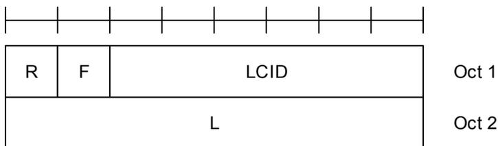
Figure 6.1.2-1: R/F/LCID/L MAC subheader with 8-bit L field
