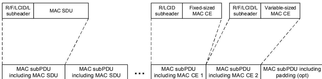
Figure 6.1.2-5: Example of a UL MAC PDU
