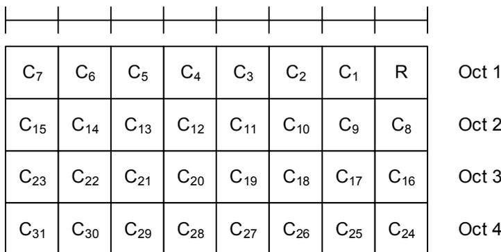
**Figure 6.1.3.10-2: SCell Activation/Deactivation MAC CE of four octets**
