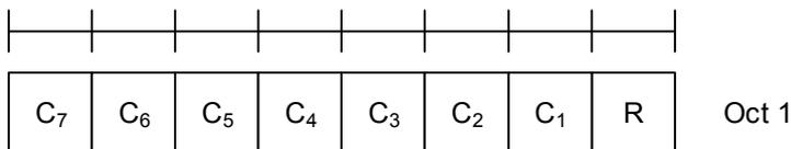
**Figure 6.1.3.10-1: SCell Activation/Deactivation MAC CE of one octet**
