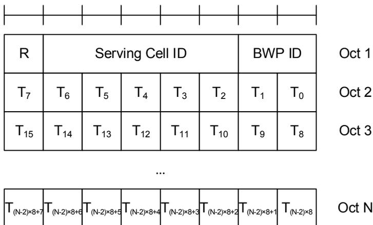
Figure 6.1.3.13-1: Aperiodic CSI Trigger State Subselection MAC CE
