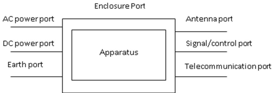
**Figure 3.1-1: Examples of ports for *hybrid AAS BS***
