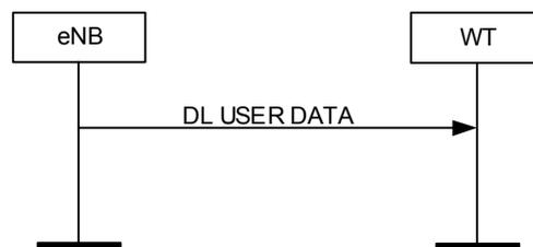
**Figure 5.4.1.1-1: Successful Transfer of Downlink User Data**
