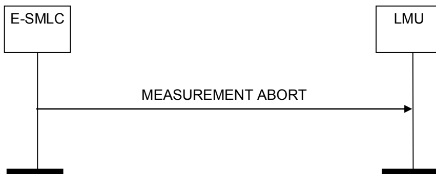
Figure 8.2.3.2.1: Measurement Abort Procedure: Successful Operation.
