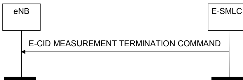
Figure 8.2.4.2-1: E-CID Measurement Termination procedure, successful operation
