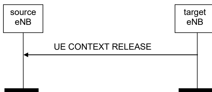
Figure 8.2.3.2-1: UE Context Release, successful operation
