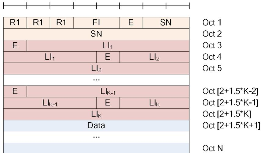
Figure 6.2.1.3-6: UMD PDU with 10 bit SN (Even number of LIs, i.e. K = 2, 4, 6, ...)
