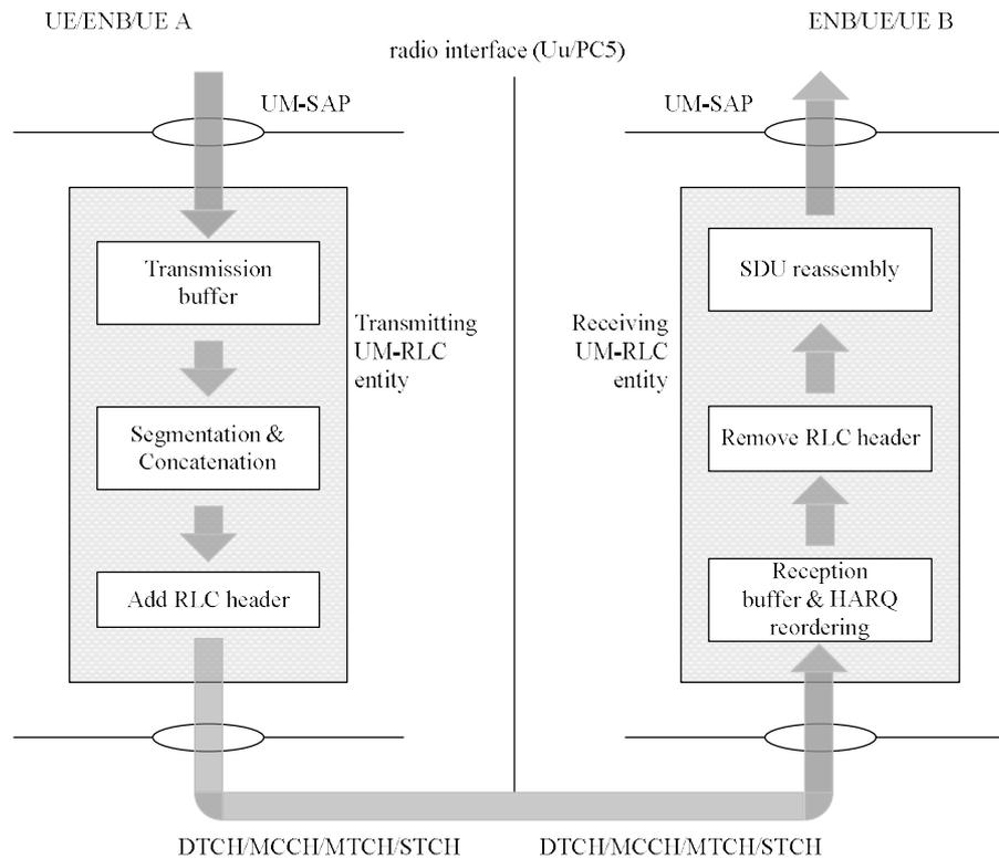
**Figure 4.2.1.2.1-1: Model of two unacknowledged mode peer entities**
