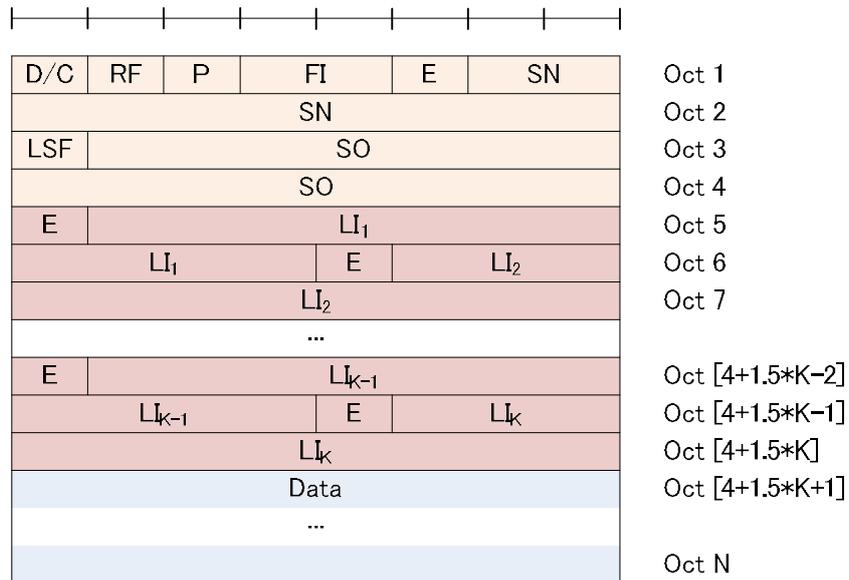
Figure 6.2.1.5-3: AMD PDU segment with 10 bit SN (length of LI field is 11 bits) (Even number of LIs, i.e. K = 2, 4, 6, ...)
