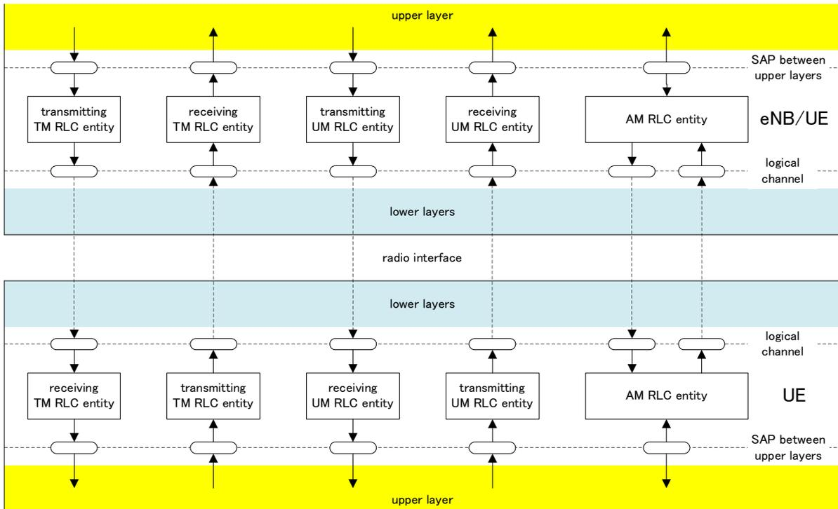
**Figure 4.2.1-1: Overview model of the RLC sub layer**
