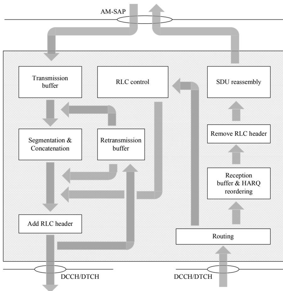
**Figure 4.2.1.3.1-1: Model of an acknowledged mode entity**
