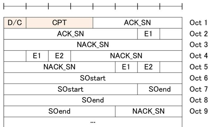
Figure 6.2.1.6-1: STATUS PDU with 10 bit SN
