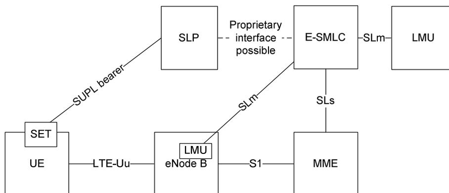
Figure 5-1: UE Positioning Architecture applicable to E-UTRAN
