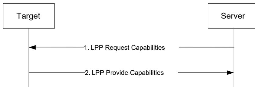
**Figure 7.1.2.1-1: LPP Capability Transfer procedure**
