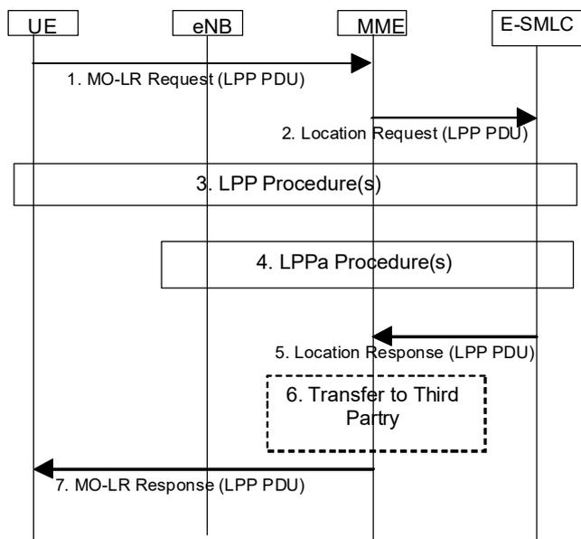
**Figure 7.3.2-1: UE Positioning Operations to support an MO-LR**
