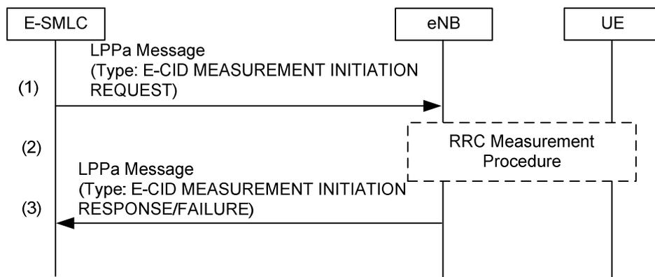
**Figure 8.3.4.3.1-1: E-SMLC-initiated Position Measurement Procedure**
