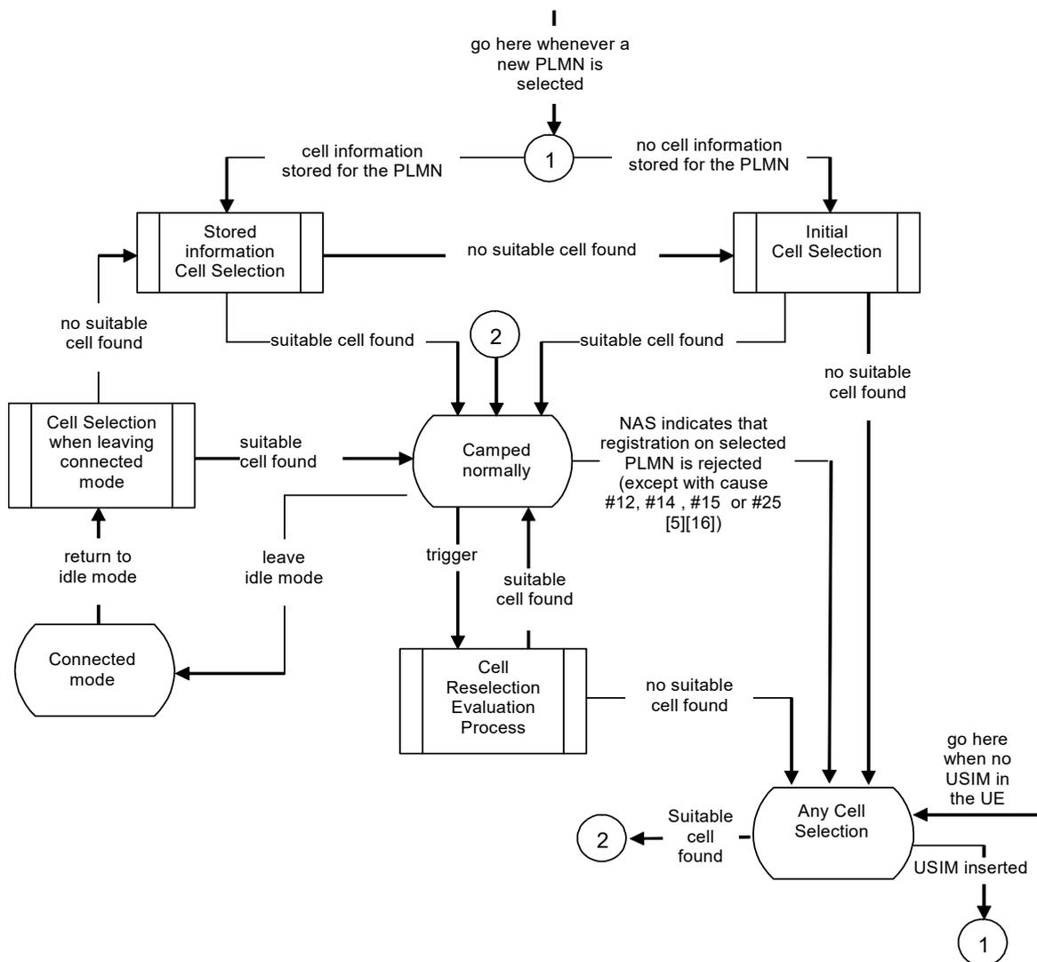
Figure 5.2.2-2: RRC\_IDLE Cell Selection and Reselection for NB-IoT
