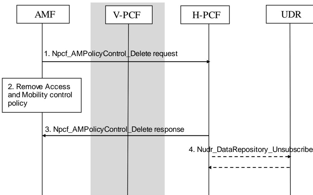
**Figure 5.1.3.1-1 AMF-initiated AM Policy Association Termination procedure**
