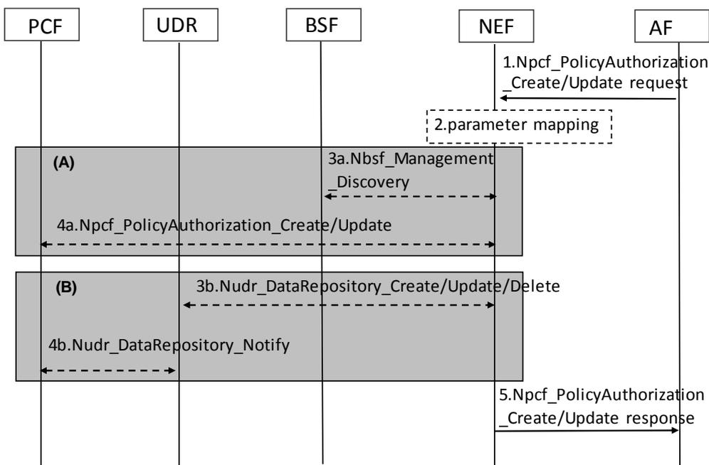
**Figure 5.6-1: AF request handling via NEF procedure**
