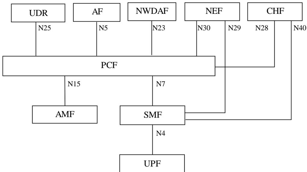
**Figure 4.1-1b: Overall non-roaming 5G Policy framework architecture (reference point representation)**
